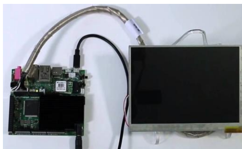
Figure 4: UDOO 7” inch Touch Screen connected to UDOO Quad board.
