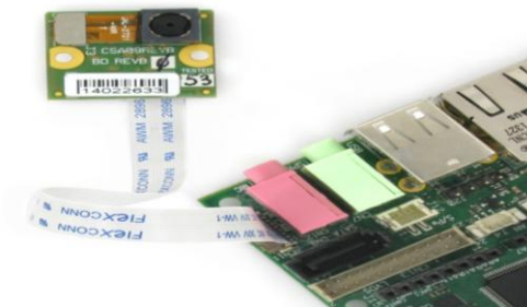
Figure 3: UDOO camera module connected to UDOO Quad board.
