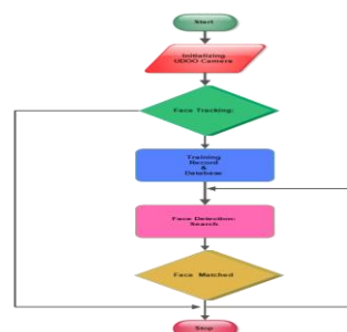
Figure 8: Flow chart of the Face Recognition system using UDOO Android
