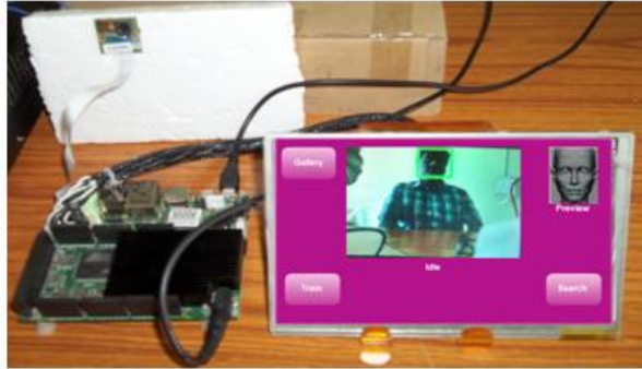
Figure -9: Shows complete experimental setup of the FRS
